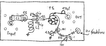
Q1: MGF 1200, 1202, 1400 1402, NETZO89, etc ie: most any GaASFET works
