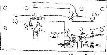
1296 MHz ULTRA LOW NOISE GAASTET Preamplifier BY E.R. "CHIP" ANGLE NGCA
